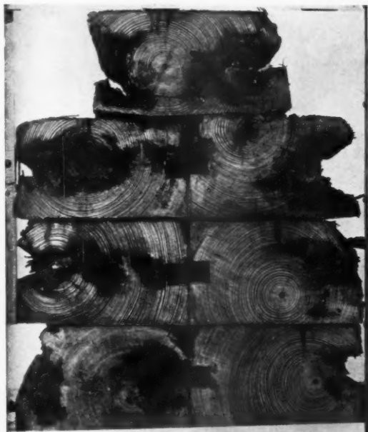
Fig. 1. Four inch longleaf pine roof planks, rotted through the centre, taken from a paper mill in Maine.
