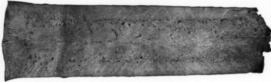
Split Ingot, Showing Blowholes
