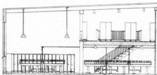
Section BB of Wash and Locker Room.
