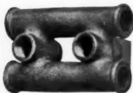
Galvanized malleable iron mixing faucet connection; right and left hand threaded, and so arranged that the hot water is at left hand side and cold water at right hand side, when double mixing faucets are attached to both sides of the fitting
