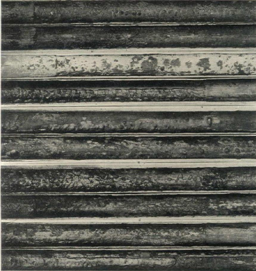
Tests by The Pittsburgh Testing Laboratory, showing the corrosive effect of untreated hot water on six steel and four wrought iron pipes.
