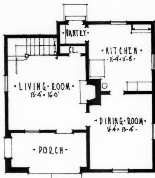
FIRST FLOOR PLAN SIX-ROOM HOUSE, TYPE E-1
