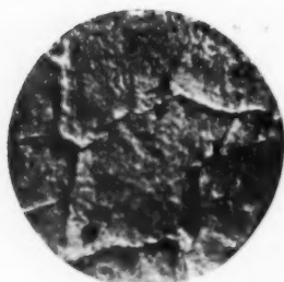
FIG. 1 White lead paint, showing chalked condition.
