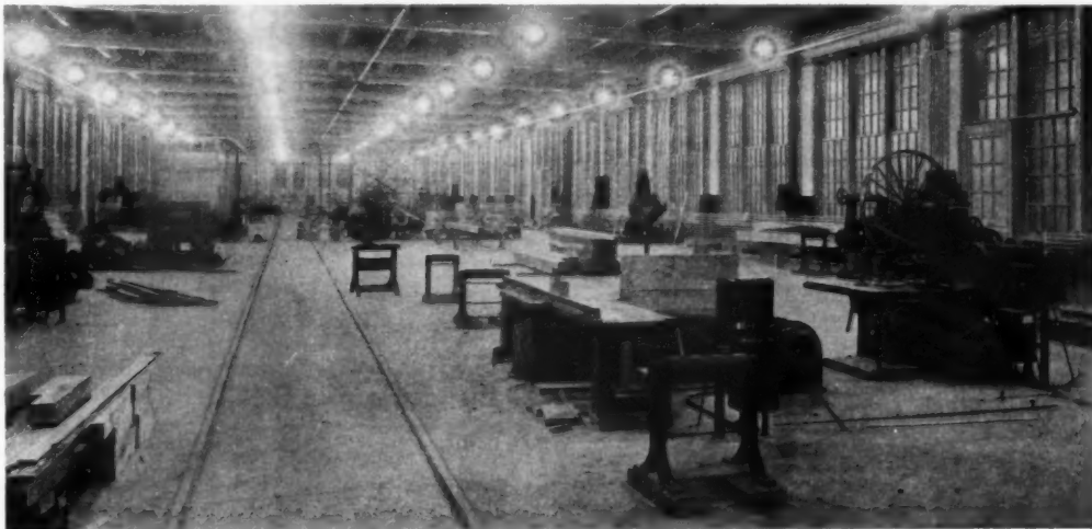
A PLANING MILL WITH 250-WATT LAMPS ON A 16-FT. MOUNTING.
