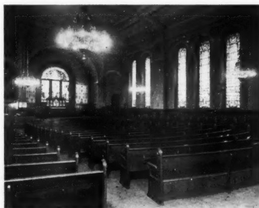
Fig. 1.—That proverbial feeling of drowsiness is not always caused by the spoken word. Exposed lights in the visual field impose a great burden upon optical controlling muscles followed by a reflex which inspires sleep through sheer fatigue. And the removal of lamps and their equipment from direct lines of vision does not always improve conditions, since reflected light, entering the eye at too acute an angle with the horizontal, is exceedingly irritating.
