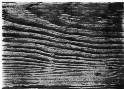
FIG. 1. NORTH CAROLINA PINE SHOWING SHRINKAGE BETWEEN RESIN LAYERS
