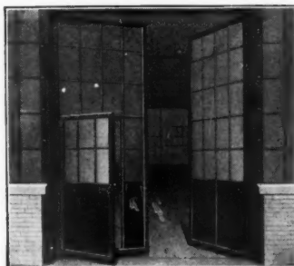
Steel channel doors for exterior or interior use. Do not warp, shrink or stick, and are fire-resisting. Corners extra strong, and machine riveted to trim. Lower portion of door filled with steel kick plate. Upper part of small wired glass lights.
