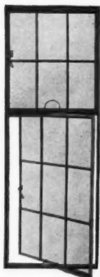
Sash vertically pivoted designed to give maximum ventilation. May be swung at 180 degrees or set at any angle to deflect air currents into building.
