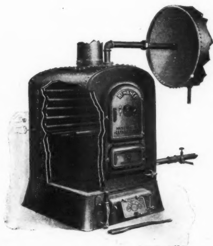
Kewanee Water Heating Garbage Burner Type D. Made in sizes to heat from 500 to 1800 gallons of water, a 50 degree raise, every hour. Other sizes and styles heat from 200 to 2600 gallons, 50 degree raise hourly.
