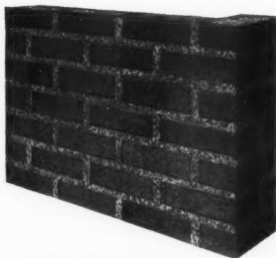
E—ROUGH-CUT FLUSH JOINT
