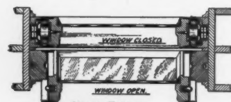
SECTION THROUGH PIVOT AND PIVOT BOLTS SHOWING FLANGES
