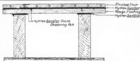
Hydrex-Saniflor Sound-Deadening Felt. As Used in Floors.
