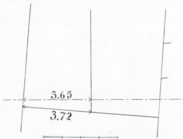
Diagram of DeFleury's sixth-story plumb in 1859, showing the difference of measures on the same plumb as taken to level and as taken to slope. (This level line in DeFleury's original survey starts from the upper step on the north side of the exterior platform and is the level which shows on the south exterior side the total dip at the base of m. 1,525.)
