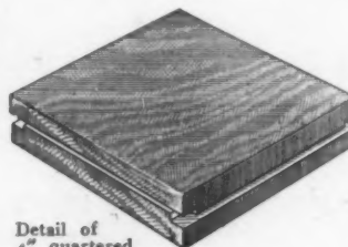
Showing two border and wall strips with bridge over compression space and short dovetailed pieces of wood to which border strips are lightly nailed.
