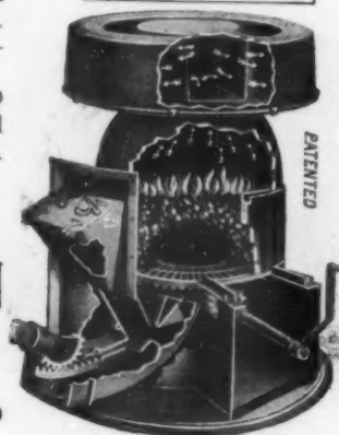
Illustration shows furnace without casing, cut away to show how coal is forced up under fire, which burns on top.
