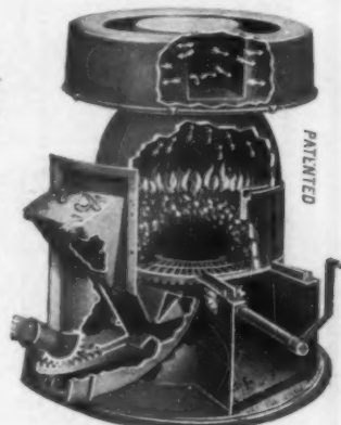
The Underfeed Furnace with casing removed, cut away to show how coal is forced up under fire, which burns at top.
