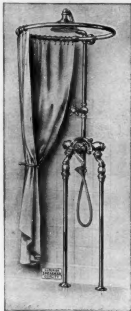
Figure 1006, Speakman Shower, with No. 1 Non-Scalding Regulating Valve, Strainer Unions, Shampoo, 24 in. x 30 in. oval curtain ring and 1/2 in. supply pipes to floor.
