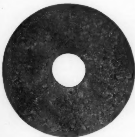
Cross Section of Nonpareil Cork Pipe Covering
