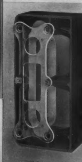
The Reinforcing Block and Turret
