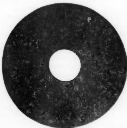
Cross Section of Nonpareil Cork Pipe Covering
