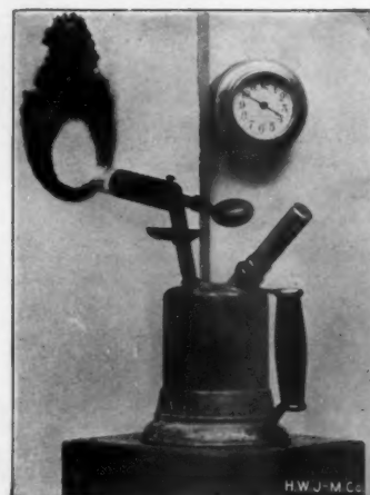
In this test the flame of a powerful blow torch was placed within two inches of J-M Asbestos Roofing. At end of fifty minutes the roofing was not burned or injured, being only slightly blackened with smoke.
