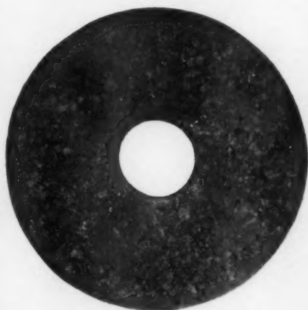
Cross Section of Nonpareil Cork Pipe Covering
