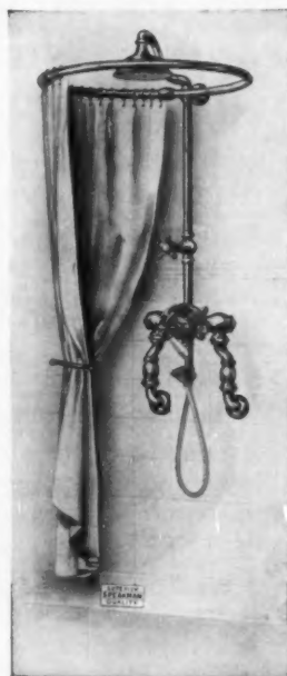
Fig. 1009 Speakman Shower, with No. 1 Non-Scalding Regulating Valve, Strainer Unions (to prevent sediment from getting into the valve or needle head), Shampoo, 24"x30" Oval Curtain Ring, White Duck Curtain and supply inlets to wall, $45.50. This shower can set over the regular bath tub.
