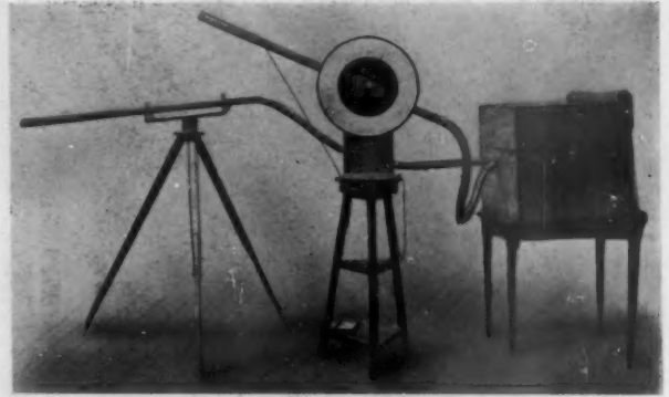
LYONS SMALL APPARATUS FOR ASCERTAINING THE POSITION OF ACOUSTIC REFLECTING POINTS
