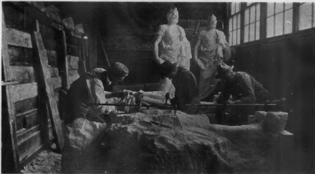
MARBLE CUTTER USING THE MEASURING MACHINE TO REDUCE THE BLOCK OF MARBLE TO EXACT PROPORTIONS OF PLASTER MODEL
