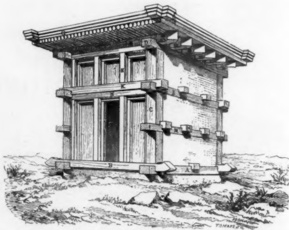
RESTORATION FROM TOMBS OF STONE of a typical house of hewn timber in ancient Lycia, Asia Minor.
