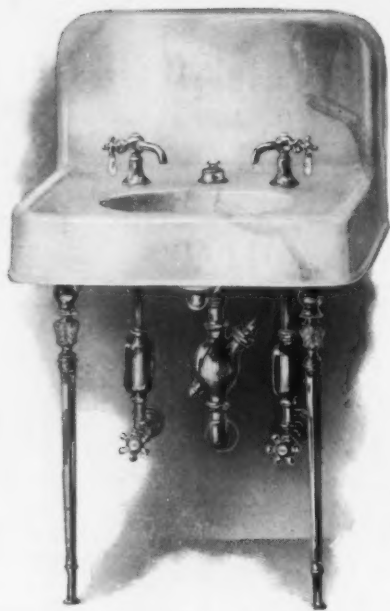
"Standard" PLATE P. 510 Porcelain Enameled "Ophir" Design Lavatory, with slab, apron, bowl and back, all in one piece, nickel-plated "Hexagon" pattern legs, "Torrance" pattern, fuller faucets with china handles and indexes, supply pipes with globe air chambers and compression stops with china indexes, Imperial waste with china index, and unique trap with waste and vent to wall.
