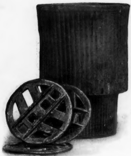
CORRODING POT FOR MAKING WHITE LEAD.
