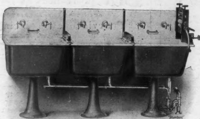
"Standard" Plate P-1285 Porcelain Enameled Flat Rim Laundry Trays, with 12-inch Porcelain Enameled Backs, Nickel-plated Union Strips with Hardwood Wringer Holders, Nickel-plated Soap Dishes, Waste Plugs, Couplings and Rubber Stoppers, Nickel-plated Fuller Adjustable Flange Bibbs, Continuous Waste and Vented "S" Trap.
