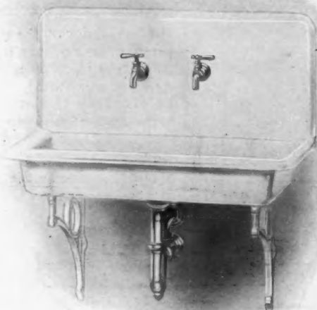
"Standard" Plate P-1206, Porcelain Enameled Roll Rim Sink and 15-inch Porcelain Enameled Back, with Brackets, Concealed Galvanized Air Chambers, Nickel-plated Strainer, Fuller Adjustable Flange Bibbs, and "P" Trap with Waste and Vent to Wall.
