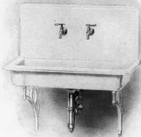
"Standard" Plate P-1206, Porcelain Enameled Roll Rim Sink and 15-inch Porcelain Enameled Back, with Brackets, Concealed Galvanized Air Chambers, Nickel-plated Strainer, Fuller Adjustable Flange Bibbs, and "P" Trap with Waste and Vent to Wall.
