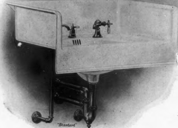
"Standard" Plate P. 545 Porcelain Enamelled "Recess" Design Lavatory, with Slab, Bowl, Overflow, Back and Ends all in one piece, Nickel-plated "Torrance" pattern Fuller Faucets with China Handles and Indexes, Supply Pipes, Keystone Waste with China Handle and "P" Trap with Waste and Vent to Wall. Designed for use in Alcoves, Closets and Wardrobes in offices, hotels and other public buildings.
