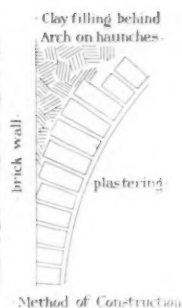
Method of Construction
