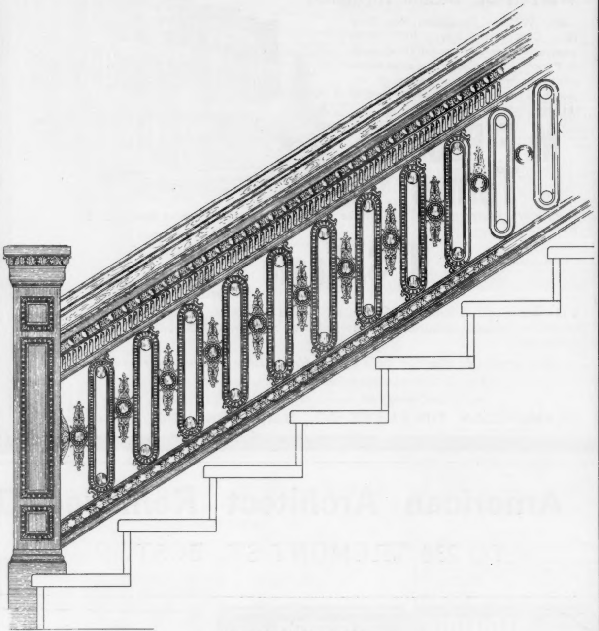
CAST IRON STAIR RAILING
