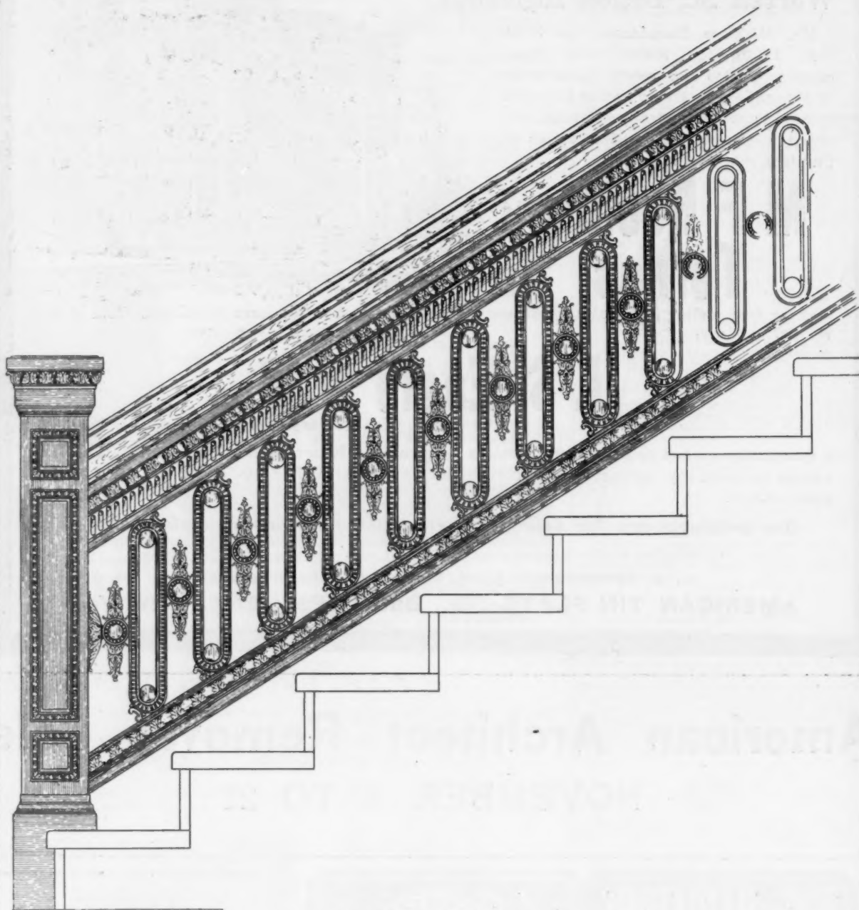
CAST IRON STAIR RAILING
