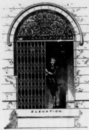
No. 1284. PITT-BOSTWICK FOLDING GUARD FOR VESTIBULES.
