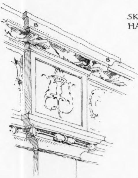
DETAIL OF CORNICE
