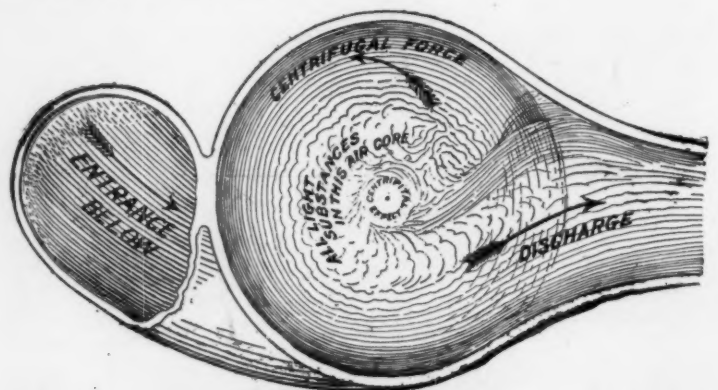
Sectional cut of "Ideal" Centrifugal and Centripetal Trap, showing the currents of water and air core formed when the Trap is in motion.
