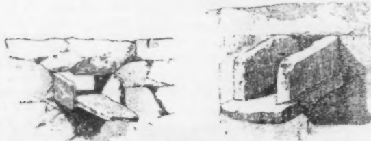
Trough Roof-drains of Stone.
