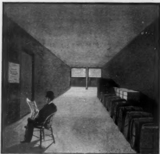
ONE-HALF BASEMENT, 170 LAKE ST., CHICAGO. BASEMENT LIGHTED BY LUXFER PRISMS. MAN READING 75 FEET FROM FRONT.
