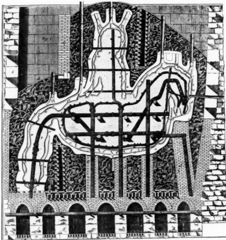
Section of Mould and Kiln for casting Bouchardon's Statue of Louis XIV. From Diderot's "Encyclopédie."
