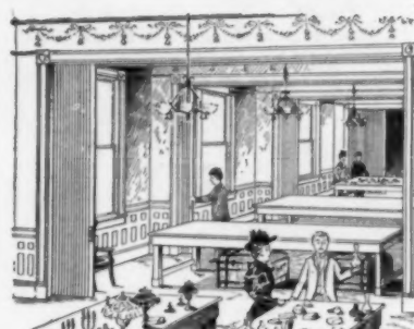
FLEXIBLE PARTITIONS SUB-DIVIDING HOTEL BANQUET HALL INTO SEVERAL SAMPLE OR DINING ROOMS.
