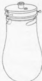
Fig. 69. Vapor-tight Globe to cover Lamp and Socket.
