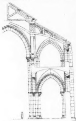
Fig. 2. Transverse Section of the Porch of the Church of Vézelay.
