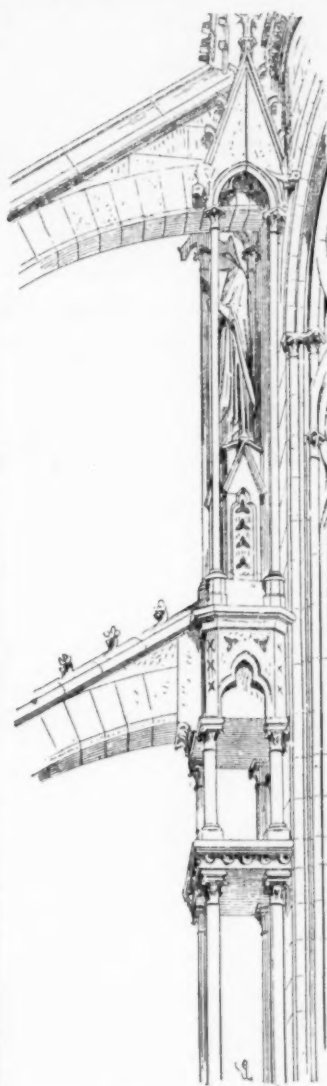
Fig. 101c. Flying-Buttresses, Choir of Beauvais Cathedral.
