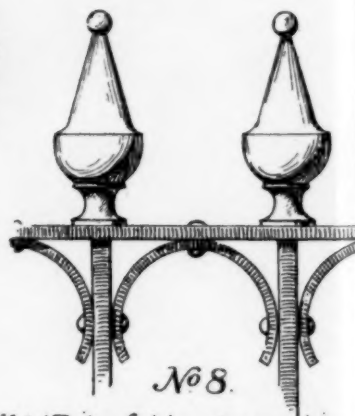
No. 8. Metal Railing-finials; showing Lines of Shade of Spheres, Cones, and Scazzos
