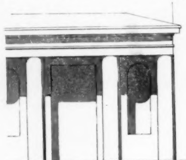
Fig. 100. Shadow of architrave shows true section of porch doorway and niches
