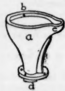
Fig. 163. Maddock's Hopper. a, Bowl. b, Flushing-rim. c, Outlet. d, Projecting lip.
