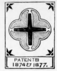
Cast or Wrought Iron, protected by gores of Porous Terra Cotta, or Lime of Teil Concrete.
