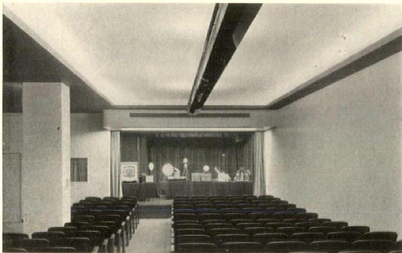
*A conference room in the General Electric Company Building, New York City—Hood & Foulhoux, architects. The trough fixture running down the middle of the ceiling is that shown in detail on the previous page. In a gun-metal mirror trough the neon and mercury vapor lamps produce a visually white light as well as varied color combinations. The scheme was conceived by A. L. Powell, illuminating engineer, and executed by the A. Ward Hendrickson Co., Inc.*
