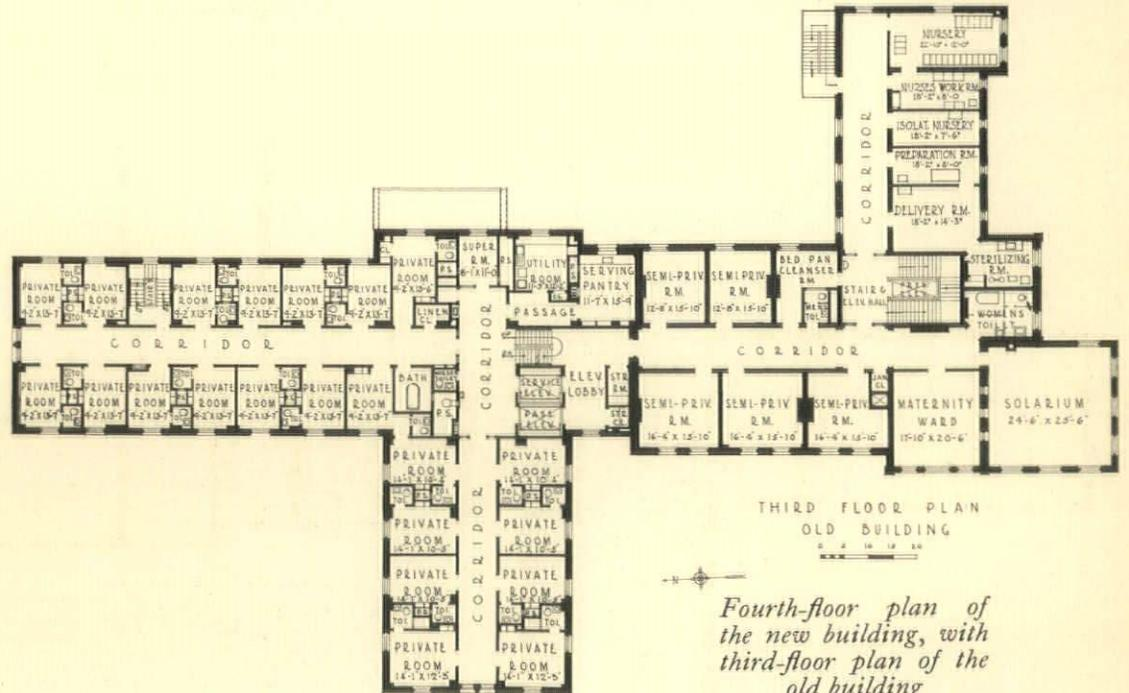
Fourth-floor plan of the new building, with third-floor plan of the old building
