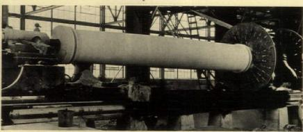
In the photographs above, two operations of machining are pictured: at the left, cutting a straight run of mouldings; and at the right, cutting mouldings on a curve where the stone is rotated against a stationary cutting tool. This machining process is accomplished by cutting edges of steel used with wet abrasives. The latter are sand, shot, chat (ground flint), depending upon the surface effect desired
