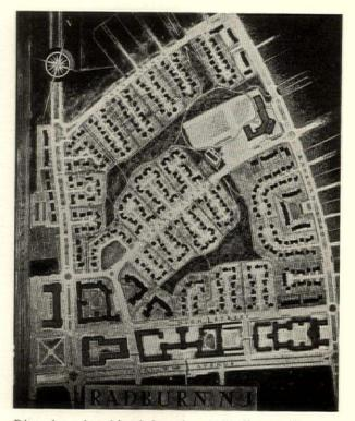
Plot plan of residential section at Radburn. Here are shown the safety-street plan and the arrangement of house groups on closed-end streets. Clarence S. Stein and Henry Wright, architects associated
