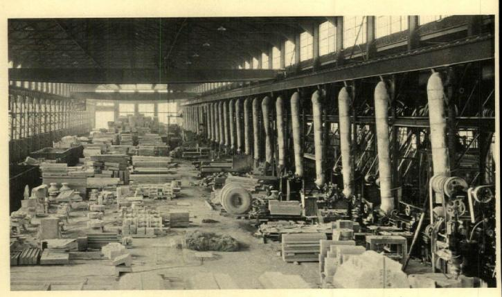
A cut stone mill, where the problem is one of arrangement so as to necessitate the fewest possible number of handlings, most of which are made with the overhead travelling crane
