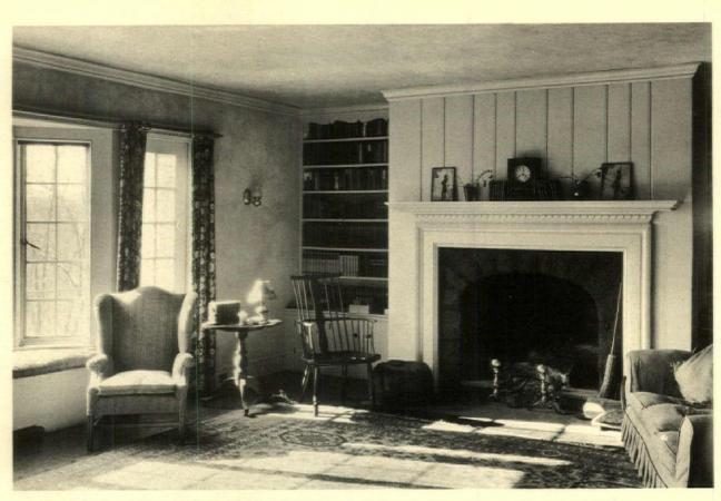
Two views of the living-room. Virtually the whole south side of this room is taken up by a range of casement windows. The fireplace is faced with native stone. Walls are of sand-finish plaster, tinted buff. All the woodwork is cream
