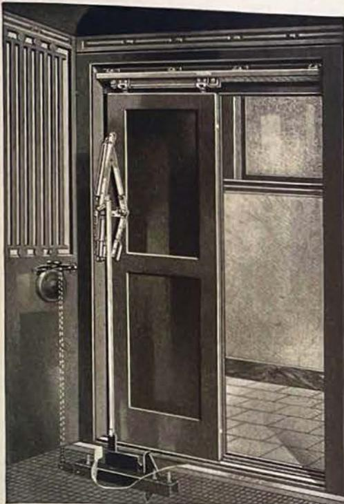
When doors are open the lock plate of the Mechanical Interlock is thrown forward and around handle of the car controller, which positively locks it, and prevents operation of the car.
