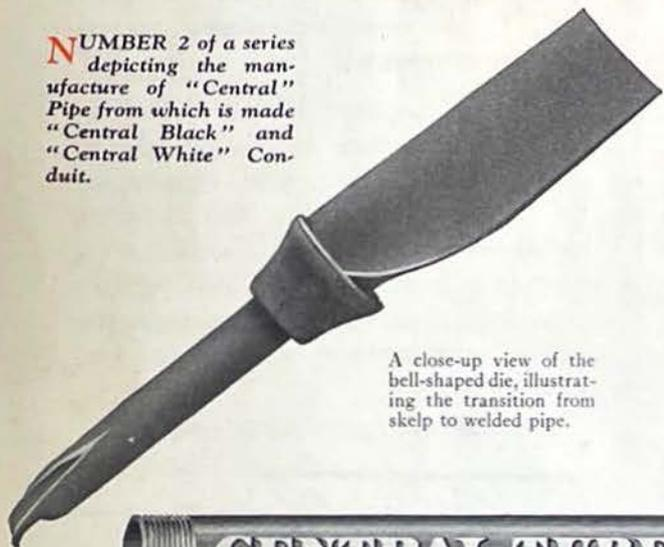
A close-up view of the bell-shaped die, illustrating the transition from skelp to welded pipe.
