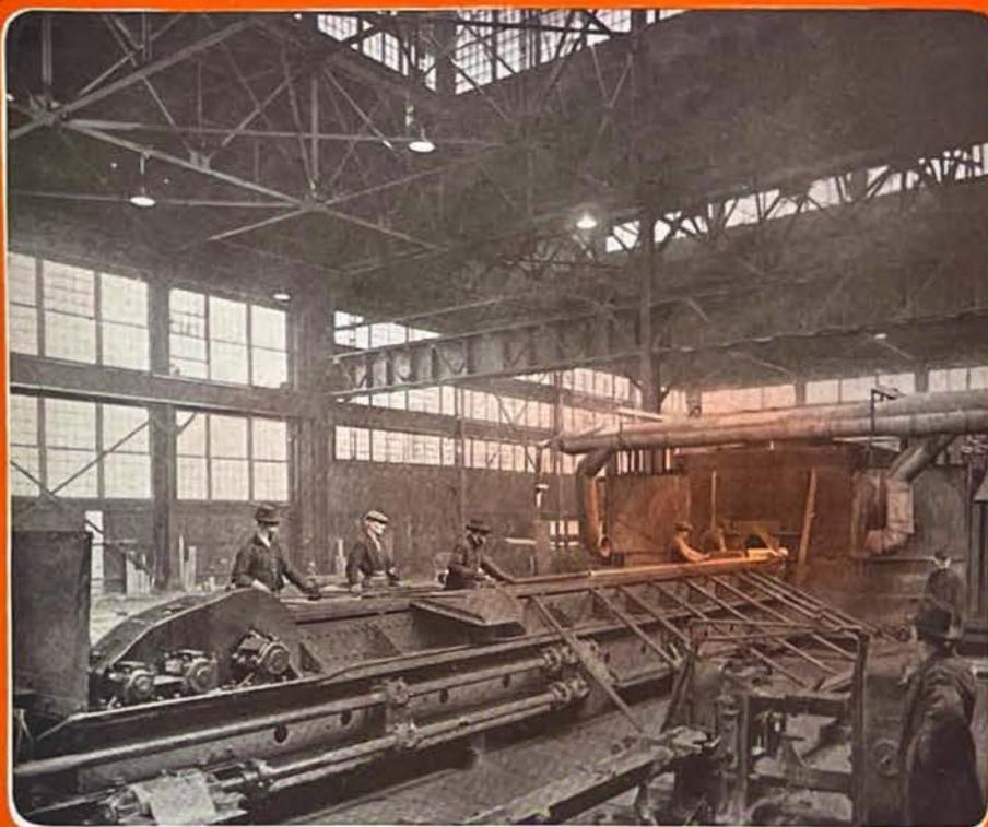
*Drawing and Welding Skelp into "Central" Pipe*
