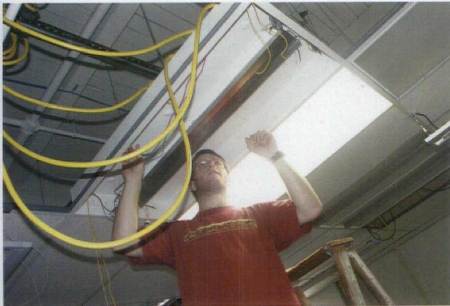
Students in the new lighting laboratory at Penn State University acquire hands-on experience with the benefits of DALI technology. Testing the functionality of a DALI control system involved retrofitting the standard electronic ballast used by the fixture with DALI-based ballasts.
