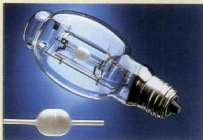
technology to provide improved color consistency, high efficacy and a CRI of 94 for high-wattage HID applications. The entire Metalarc Powerball Ceramic family of lamps incorporates Metalarc Pro-Tech technology where a protective shroud around the arc tube allows the lamps to be used in open fixtures. **Circle No. 110**
