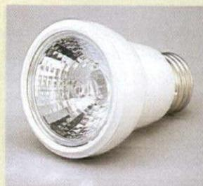
**GE Lighting** has introduced the Diamond Precise Electronic Compact Reflector, a screw-base MR16 featuring built-in electronics that convert from line voltage to 12V. Operating at 12W, Diamond Precise can replace 50W PAR20 and 50W R20 lamps and delivers 13.8 lumens per watt and 5,000 hours of life. Lamps measure 3/16 in. in diameter and are available for spot- and floodlighting. Color temperature is 2950K. **Circle No. 111**
