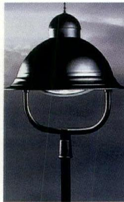
For outdoor area and roadway lighting, **Metrolux'** Town-Master Series employs a one-piece reflector assembly with a chemically brightened, clear anodized surface to maximize light output. The reflector delivers an effective projected area (EPA) of 3.4 sq. ft. and is rotatable through 360 degrees to facilitate aiming. Computer-enhanced reflector facets diffuse emitted light and redirect light away from the lamp's arc tube for safety and
