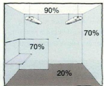
A small increase in room reflectances produces a big improvement in efficiency. The lighter room provides 55% more light on the work surface for the same energy or uses 70% less energy to provide equivalent brightness. The lighter room also provides better brightness ratios, comfort and daylight distribution.
