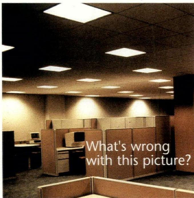
Avoid staggered layouts and locating fixtures too close to walls.
